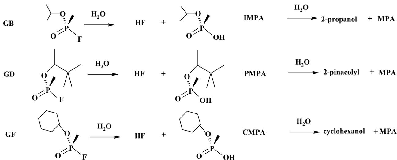
Figure 1. Hydrolysis pathways for G-Series nerve agents.
