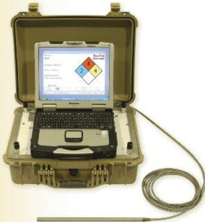
RamanID with 5 meter fiber optic probe
